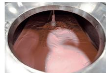
From left, the Osgood Filler machine, which packs 65 cartons per minute and puts on its safety seal and lid; large steel vats mix background base flavors, which will be blended with additional ingredients to achieve one of 500 possible varieties; and a tub of ice cream makes its way down the line for final packaging.
