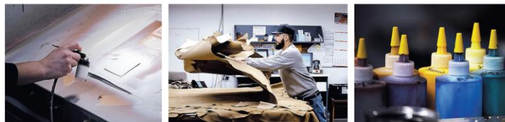
Checkwise, from top: Leather pieces are stored on horses with wheels to prevent wrinkling and give workers easy access when the orders come in at Garrett Leather in Cheektowaga. Containers hold the hundreds of dyes that are used to custom color hides for special orders. Shipping specialist Tyler Salerno flips and inspects the hides that were specifically ordered to be the surface for seating on a private jet. Colorist Carolyn Perillo uses dyes to match leather furniture that will go into the seating and trim of an aircraft in France.
